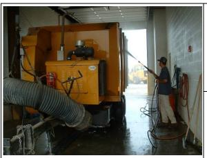
Wastes from pressure washers must be carefully managed to prevent contamination and ensure permit compliance.
