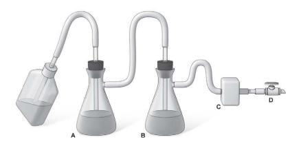
The catch flask (A) should contain disinfectant. An overflow flask (B) should be connected to this flask. A filter, with both hydrophobic and HEPA components (C), should be in place between the trap flasks and the vacuum source (D).
